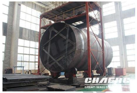
Due to transportation reasons, the rotary kiln is composed of shell segments. Because the outer circle of the kiln cylinder is not processed, the perpendicularity of the end face to the center of rotation cannot be directly measured. In the process design, the perpendicularity of the end face is converted into parallelism and the coincidence of the axes at both ends according to the structure of the cylinder.
