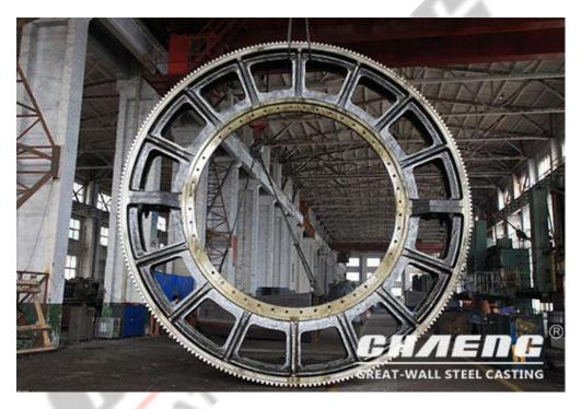
In view of the girth gear deformation problem that often occurs in cement plants, CHAENG has optimized the girth gear manufacturing process on the basis of summing up the traditional processing technology, improved process details, and greatly increased the life of the girth gear.
