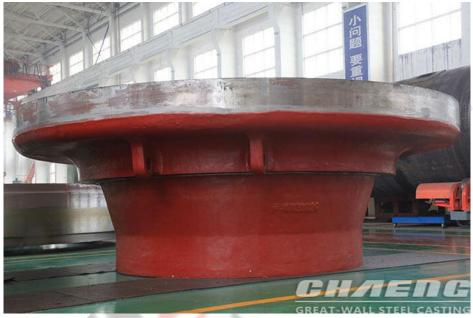
The grinding table is one of the key components of the vertical mill. It is mainly composed of the retainer ring, the lining plate and the base. CHAENG optimizes the design of the grinding table casting process to make the base of the grinding table evenly stressed, increase the bite angle between the grinding roller and the grinding table, so as to avoid the erosion of the non-wear surface of the table.
