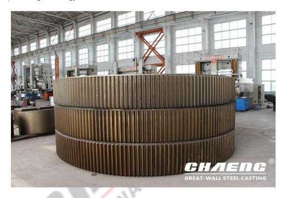
The requirements of CHAENG for the girth gear are high rotational efficiency, high power, long service life, low noise and low heat generation. In actual production, the quality requirements of large girth gears are very strict, so the processing of girth gears is very important. The following is a description of casting and processing technology of non-standard girth gear made by CHAENG.
